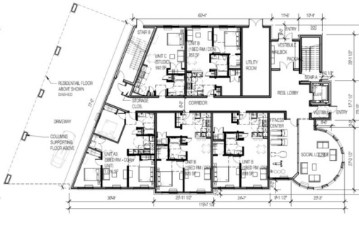
1 FIRST FLOOR PLAN SCALE: 1/8" = 1'-0"
