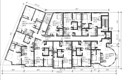
2 TYPICAL UPPER FLOORS (2ND & 3RD) SCALE: 1/8" = 1'-0"
